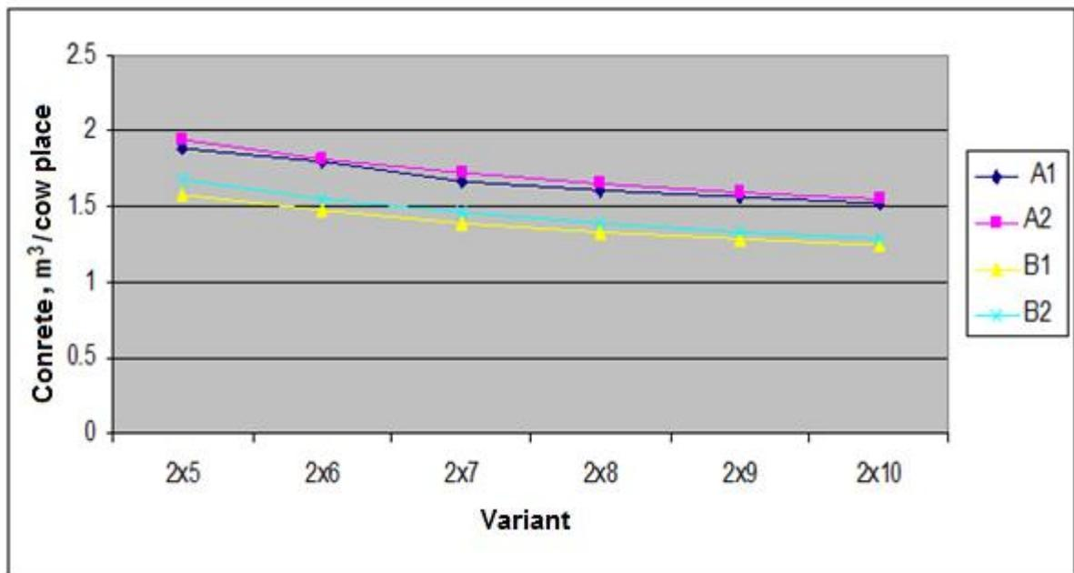
**Figure 4.** Effect of milking parlour capacity on the relative amount of concrete per cow place in a conventional exit variant
