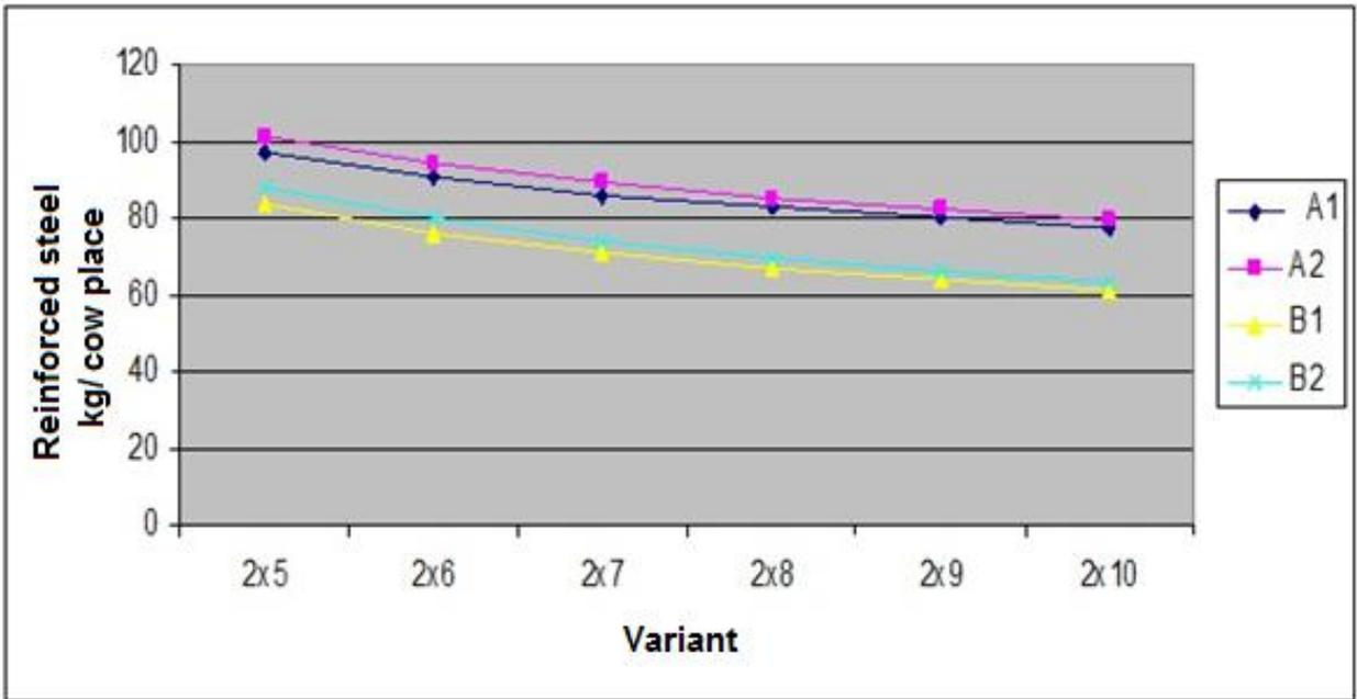
**Figure 1.** Effect of milking parlour capacity on the relative weight of reinforced steel per cow place in a conventional exit variant
