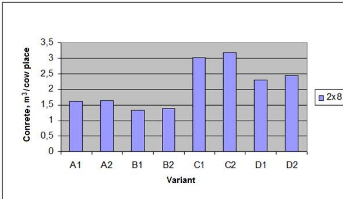
**Figure 5.** Comparative analysis of the relative amount of concrete for herringbone parlours with different positioning angle and different entry/exit variant
