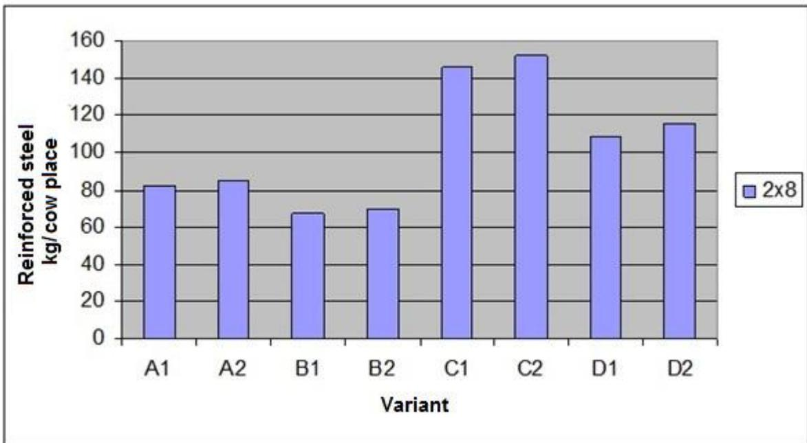
**Figure 2.** Comparative analysis of the relative weight of reinforced steel for herringbone parlours with different positioning angle and different entry/exit combination
